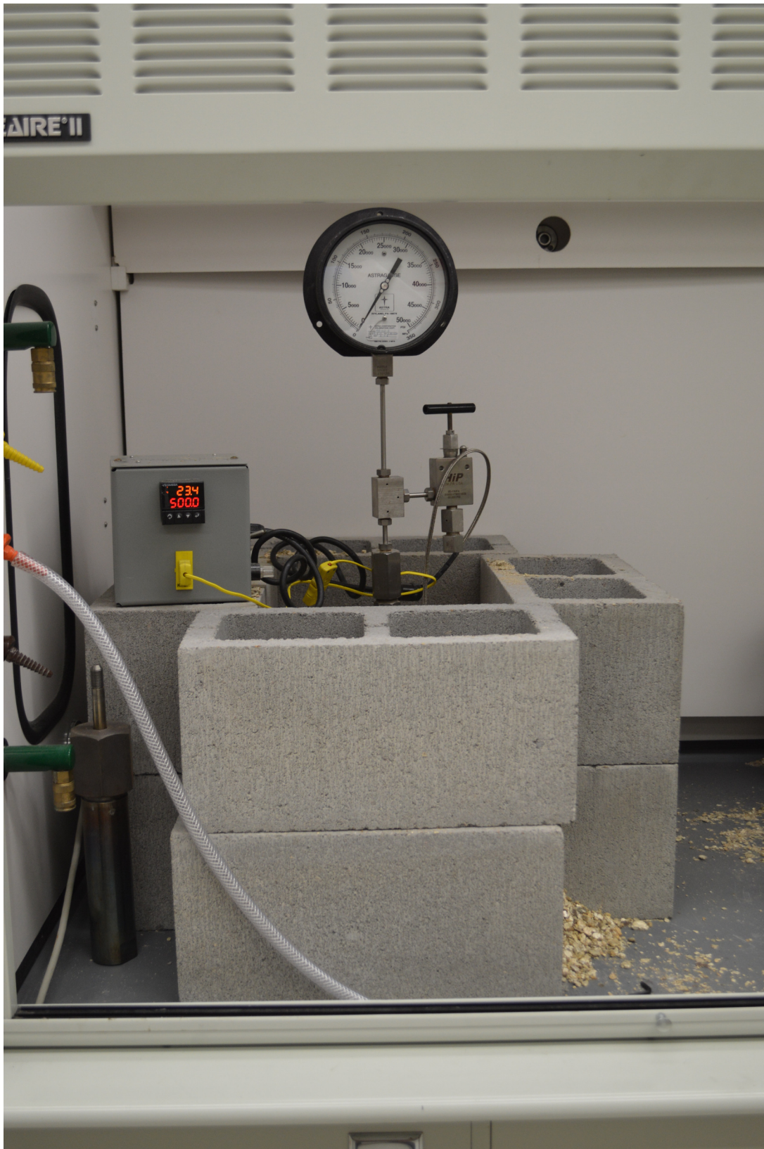
Figure A.6 Stable heating is achieved by placing the system in a pit insulated by vermiculite.
