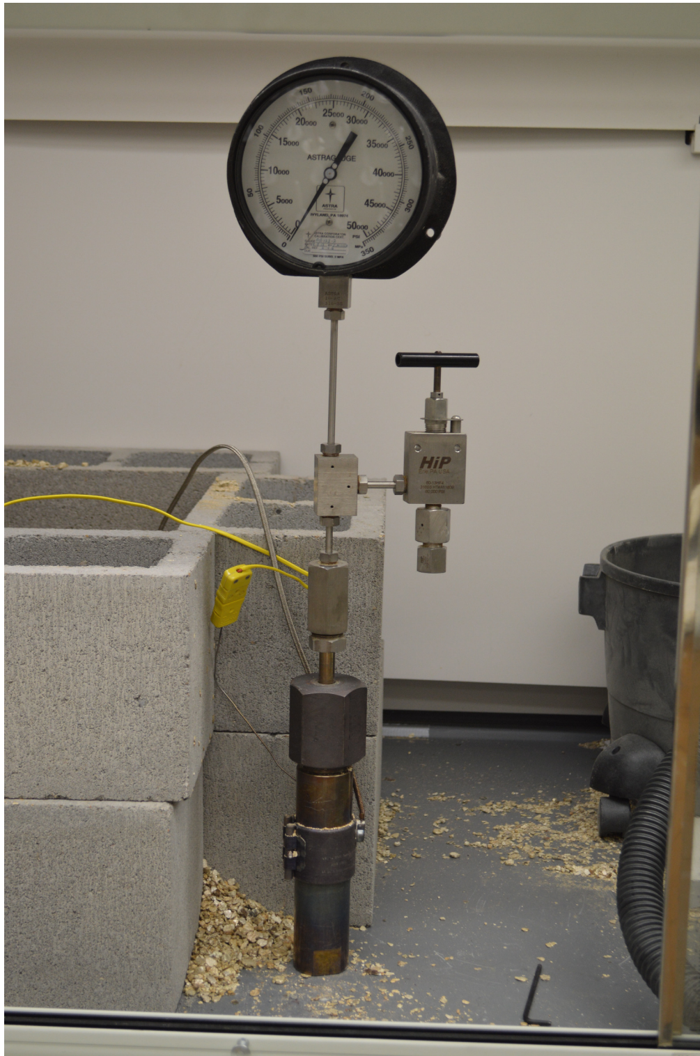
Figure A.5 The system is heated by attaching a band heater and thermocouple.
