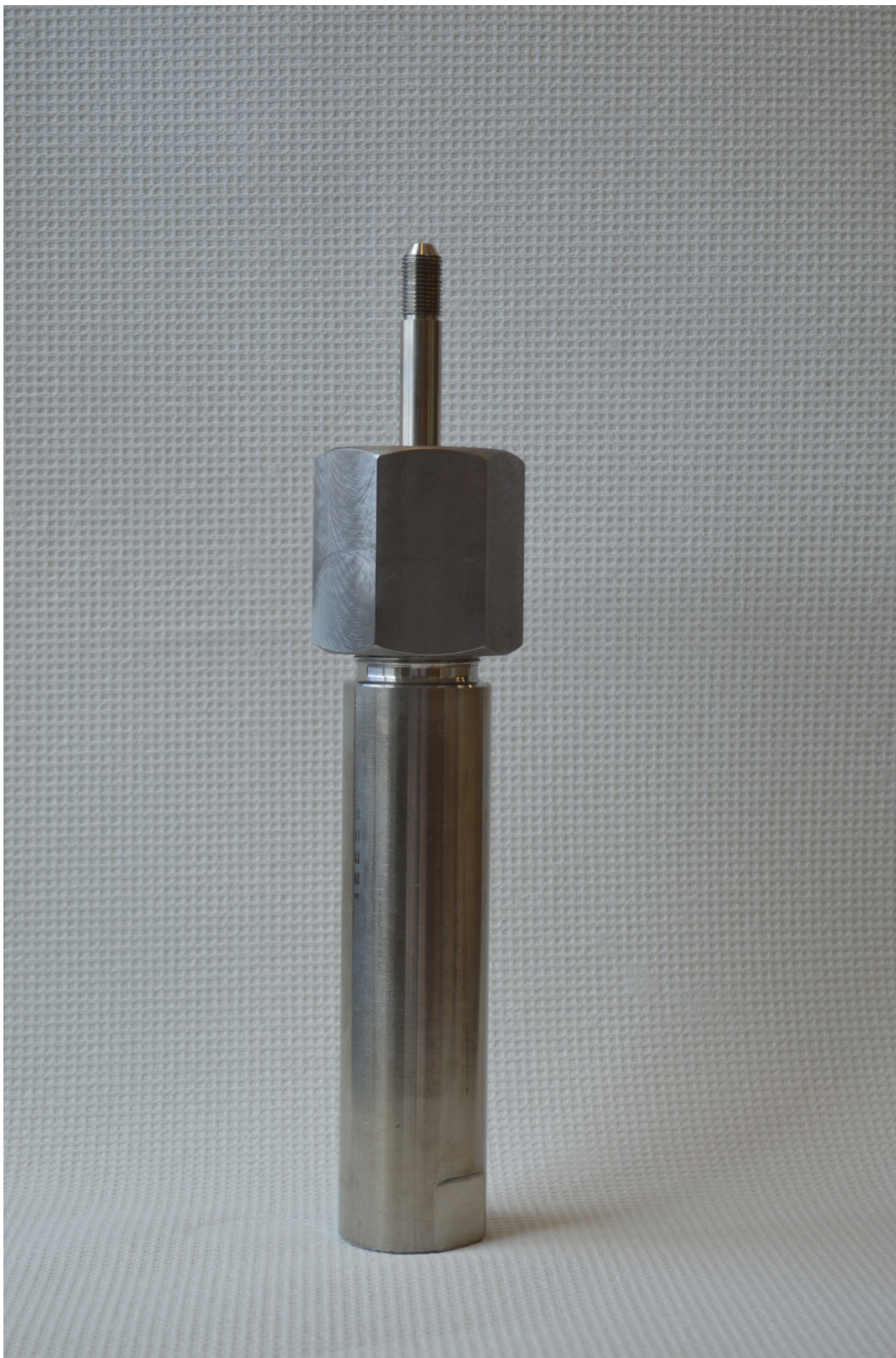
Figure A.2 Assembled the cap drives the plunger into the vessel creating a metal-metal seal. This specific type of sealing mechanism is known as a Tuttle Cold seal.
