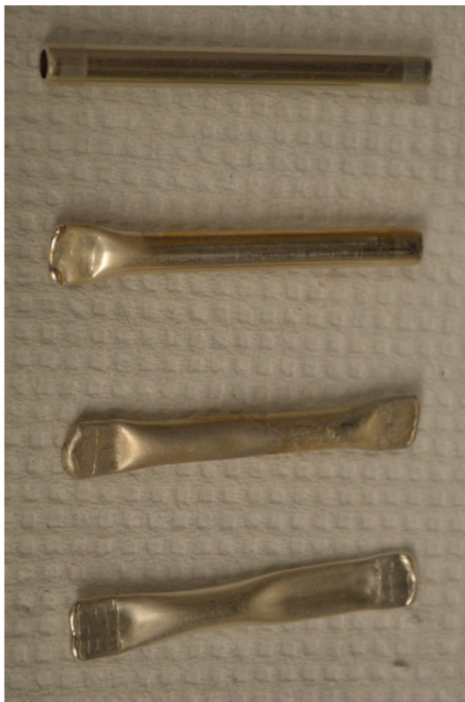
Figure A.8 Silver floating liners used for basic conditions. From top to bottom: fine silver tubing, crimped and welded, loaded and sealed, and crushed after reaction.
