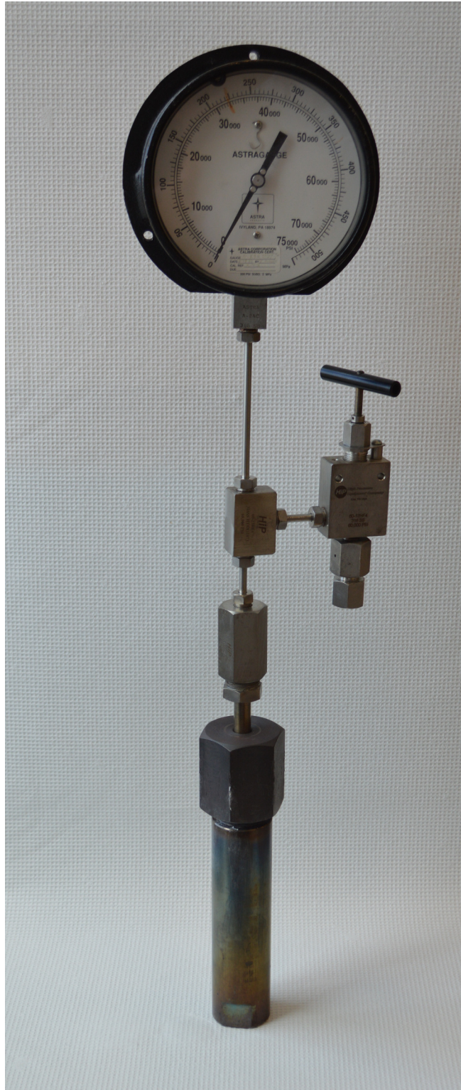
Figure A.3 A pressure apparatus is attached to monitor pressure. (In this picture the metal is more a brown color due to repeated heat-treating.)
