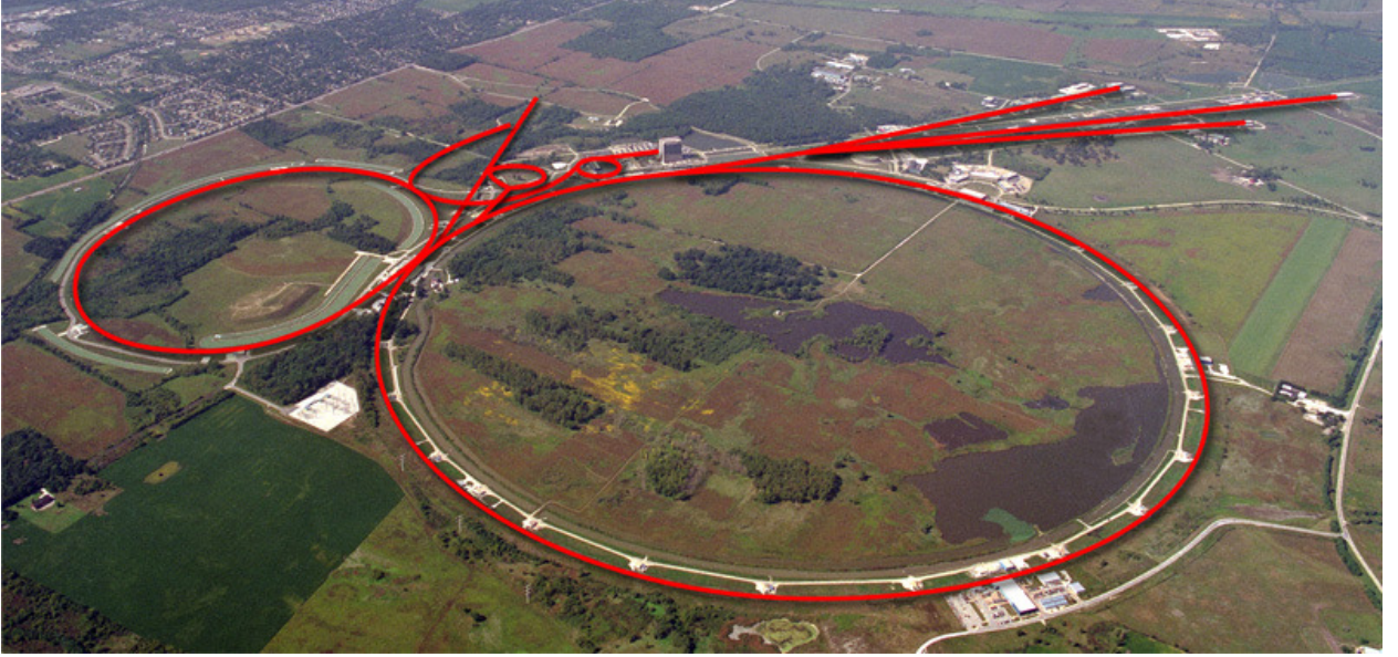
Figure 2.1: An aerial view of Fermilab, looking in the northwestward direction. The red lines show the schematic of the accelerator complex. Tevatron is the largest circle in the foreground. DØ detector is located at the building complex near the lower-right corner.
