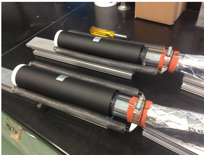
Figure B.5: The method used to attach PMT to light guides is illustrated in this photo. After the Silicon RTV was applied, the PMT/Light guide joint was held together using the device shown in this photo. Constant pressure had to be applied to the joint to ensure best results.
