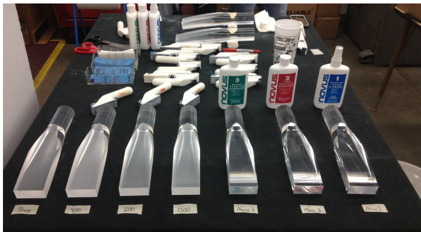
Figure B.4: An illustration of the different steps of polishing that the light guides had to go through. Several sand papers were used in the process, leading to the shades variation observed above.
