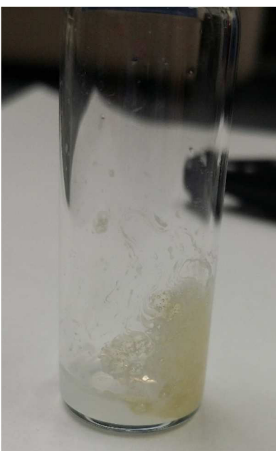
Figure 3.6 Terpolymer Swollen in 1:1 weight ratio of terpolymer:H 2 O; a turbid solution on the bottom of the vial is a polymer solution
