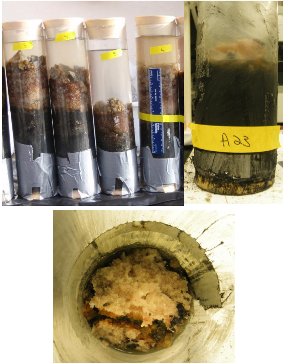
Figure 3.2. Picture of small cores from GN Pond 9 and CAL Pond 23. A. GN Pond 9. Samples were broken down into three sections to represent the visible differences in the sediment, top crustal material, middle rubble material, bottom black sediment. B. Small core from CAL Pond 23 shows the black sediment and gypsum crust that was hand-placed into the small cores; site water also was collected and placed in the small cores for transport back to NASA Ames Center.
