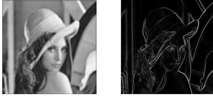
Figure 4.4: Blur-minimization Edge Detector: a) blurred image b) robust morphological gradient
