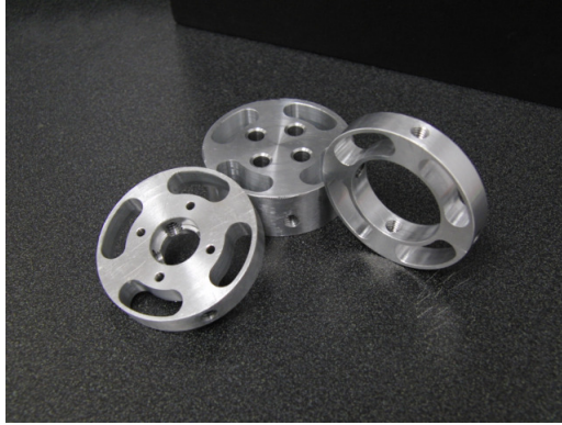
Figure 2.4: Aluminum boom inserts replaced the plastic hip seen in Fig. 2.2 by allowing the hip motor to be embedded in the boom. These parts can be seen as blue and red discs in Fig 2.5.
