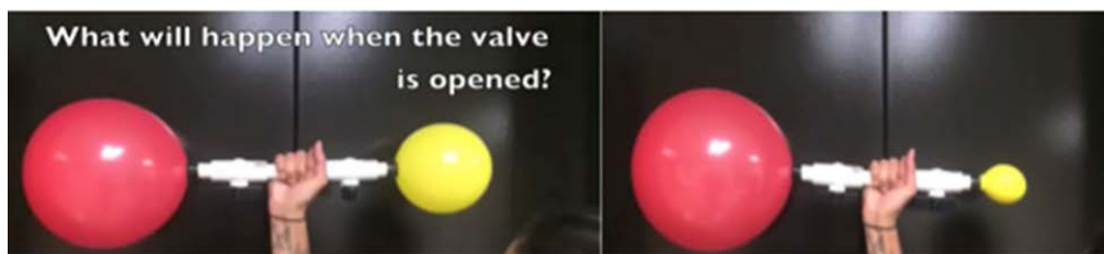
Figure 3. The two-balloon experiment, showing the relationship between pressure and elasticity in a rubber balloon.
