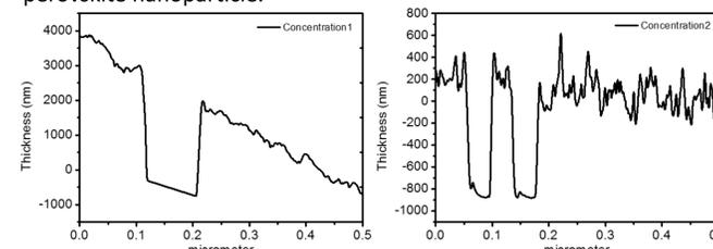
**Figure 7:** Using Atomic Force Microscopy (AFM) imaging, glass thin film thickness was determined for 2 different concentrations of the MAPbBr<sub>x</sub>Cl<sub>3-x</sub> perovskite nanoparticles. NOTE: Concentration decreases from left to right.
