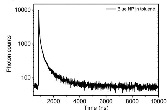
**Figure 3:** Time resolved photoluminescence decay of the blue emissive nanoparticles in Toluene.
