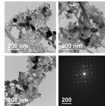
**Figure 4:** Transmission electron microscopy (TEM) images showing the sizes of the nanocrystals (10 nanometers) as well as electron diffraction (4<sup>th</sup> image).
