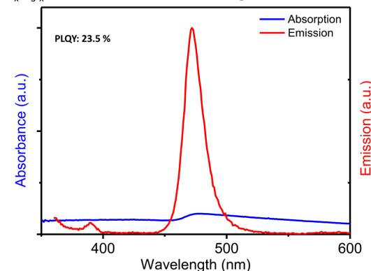
**Figure 2:** This image shows the absorption and emission spectra of a sample in Toluene, which calculated the Photoluminescence Quantum Yield (PLQY) to be 23.5%.
