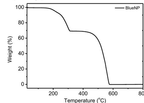
**Figure 5:** This shows the change in weight percent versus temperature using Thermogravimetric Analysis (TGA) of the perovskite.
