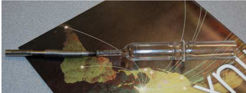
Figure 3.5: Glass channel is closed in the middle and has glass to metal seal at the top
