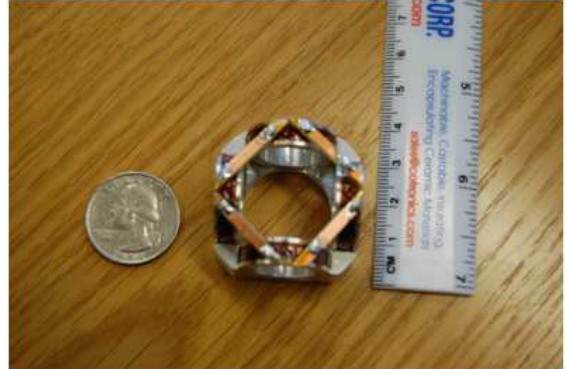
Figure 3.4: Quadruple magnet assembly
