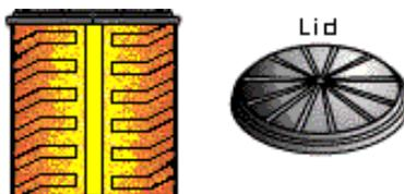
Figure 2.2: Fitch Barrel Attenuator
